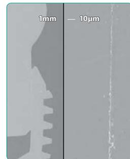
Based on a well known engineering principle, Bicon's 1.5 degree locking taper connection provides a proven bacterial seal at the implant to abutment interface, with a microgap of less than 0.5 microns. Bicon's bacterial seal avoids the microbial leakage issues that can result in inflammation of the soft tissue around an implant, which could lead to the loss of bone around the implant and even the loss of the implant itself. Bicon is the only system with a proven bacterial seal.
