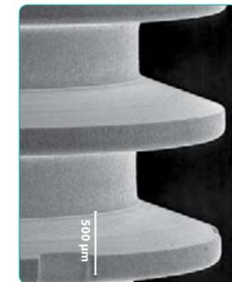
Since 1985, each Bicon implant has been grit blasted with alumina and passivated in a nitric acid solution. This innovative controlled surface is known as Integra-Ti™. Since 1988, the Bicon implant has been available with a calcium phosphate based treatment known as Integra-CP™.
